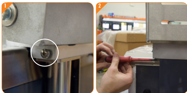
Step 8: Fix the grid frame with the short screws, washers and spring washers on both sides
