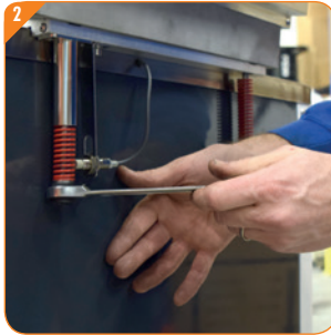
Step 4 : Mount springs on both sides and tighten screws
