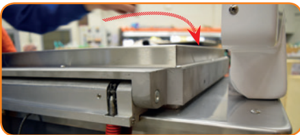
Step 6: Close the gridframe onto the machine
