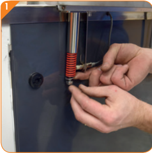
Step 4 : Mount springs on both sides and tighten screws
