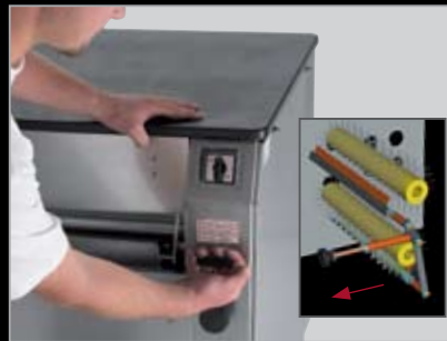
Cleaning system for the brushes
