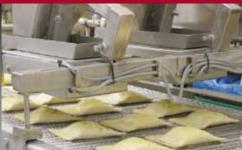
The system can be used for large Capacity of 800 - 1000 trays per hour. The trays are taken through the system and cleaned with the baking side up, which means that the trays are ready to be used right away without any need to turn
