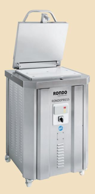
You use the Rondopress to shape consistent blocks of dough and fat plates easily and without exertion:
