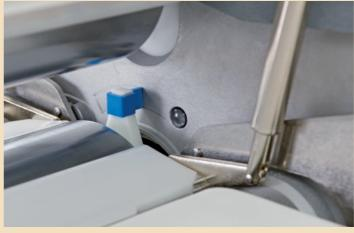
Clean photoelectric cells are a requirement for the reliable reversing of electronic dough sheeters. RONDO photoelectric cells are cleaned automatically with every pass.
