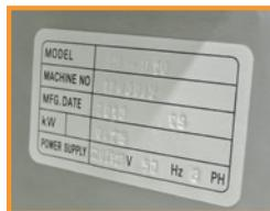
First check the manufacturer's name tag on the machine, in order to check whether the desired power supply is the same as the one that is being provided by your electricity company.
